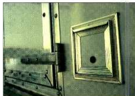
Small "rat hole" near doorway allows for cabling to enter truck without having to go through the doorway.
